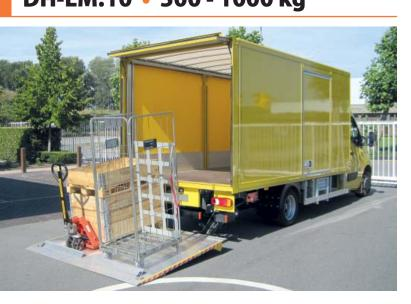
The **4-cylinder** DH-LM.10 is DHOLLANDIA's **best seller** in the light capacity lift range. Thanks to its **superior stability** and performance in comparison to competing 2-cylinder lifts, and its competitive pricing, it offers an **excellent price-quality ratio**.
