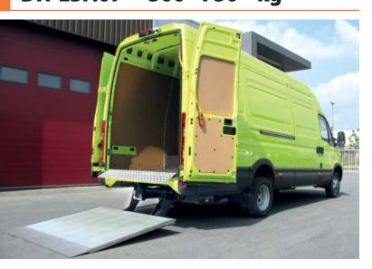
The DH-LSP.07 is a **robust lift** with maximum 750 kg lift capacity [depending on the type of vehicle (\*)].
