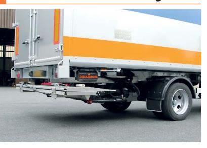
The DH-SM.15 is the **lightest of the conventional slider lifts** with single fold platforms. It is equipped with a compact lift frame and short lift arms, in order to minimize the required overhang, and forms an ideal fit for light and medium capacity trucks of 7.5 to 12T GVW.
